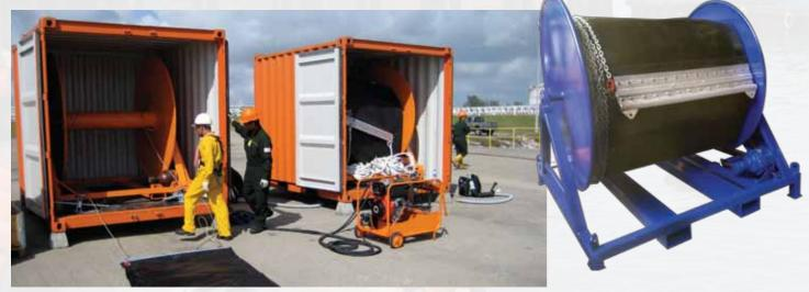
KAJ manufacture a complete range of custom-built boom reels for both the rubber boom range and the PVC/PU booms. These are either open style or built into the frame of a custom made container. All reels are driven hydraulically from our range of diesel power packs and are manufactured of steel plates and profiles and finished with a high quality, 3-layer epoxy paint system. The containers have a floor of 25mm plywood plate.
